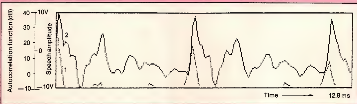
Figure E. Autocorrelation function (1) and speech samples (2) for a voiced window.
